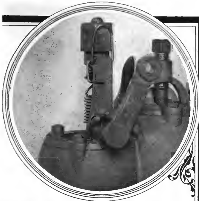
Fig. 5—Presenting the mechanism for the auxiliary air control and the lever placed to actuate the same
